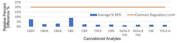
The Relative Percent Difference (RPD) for 11 individual cannabinoid analytes from seven different cannabis samples prepared using automated (**Dilution**Station) and manual methods. All RPD values were below 10%, well under the commonly accepted 20% regulatory threshold, demonstrating compliance with stringent testing requirements. 9 of the 11 analytes were within 5%, with only 2 analytes being reported as between 5 and 10%.
