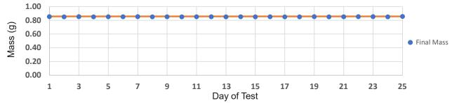
Daily QC of automated 10x dilution of cannabis extracts using **Dilution**Station over a 25-day period. After manual sonication, vortexing, and centrifugation, **Dilution**Station dispensed 100  $\mu$ L of extract with 900  $\mu$ L of 9:1 methanol/chloroform solvent directly into 2 mL HPLC vials. Gravimetric analysis showed an average recovery of 99.39  $\pm$  0.18% (0.86 g), confirming high reliability for low-volume dilutions.
