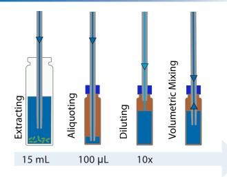
**Dilution**Station dispenses 15 mL of a 9:1 methanol/chloroform mixture to extract cannabinoids. Manual sonication, vortexing, and centrifugation complete the extraction by separating cannabinoid analytes from the plant material. A 100 µL aliquot of the extract is then diluted 10x to a final volume of 1 mL and volumetrically mixed.
